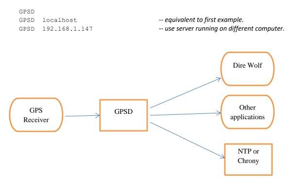
In this case, the applications don't know or care about the specifics of how GPSD is communicating with the receiver. They receive location information boiled down to a common message format.
