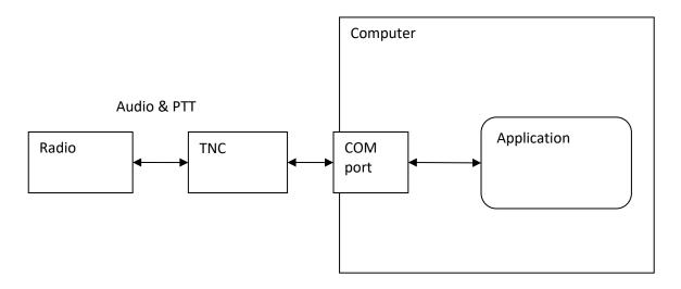
Dire Wolf is a software replacement for a separate TNC. One way of using it is illustrated below.
