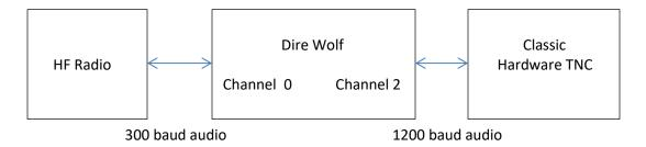
A 300 baud frame is received over the HF radio. Exactly the same thing is sent out channel 2 except at a different data rate. The TNC processes the frame and possibly sends a response. The 1200 baud packet goes into channel 2. Dire Wolf sends the same thing out to the radio, via channel 0, with a different data rate.
