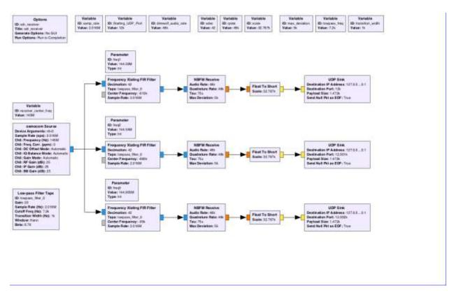
What I've routinely done is to use GnuRadio (ultimately a python script) for listening to multiple frequencies with a single SDR dongle (assuming they're all within ~2.4MHz of each other). Then have GnuRadio output that audio over a different UDP port for each frequency. That enables one to get away with just a single SDR stick, antenna, and Dire Wolf instance. Then have a Dire Wolf configured something like this:
