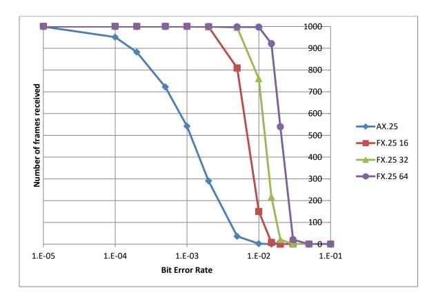
Depending on the FX.25 mode, up to 32 corrupted bytes (yes, bytes, not bits) can be corrected in a frame. Regular AX.25 fails if even a single bit gets corrupted. **FX.25 keeps going strong long after regular AX.25 is completely useless.**
