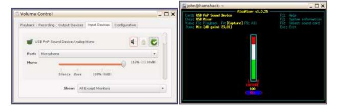
If the user has PulseAudio installed, the installing of pavucontrol is mandatory to make sure the right audio routing is done. In many respects, pavucontrol can do everything that alsamixer can do but not the other way around. Unfortunately, there are reports that pavucontrol can create blocking issues and programs will crash if it's running or they will stop running when pavucontrol is loaded.
