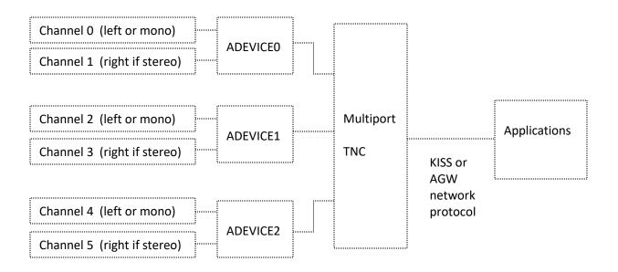
Applications use a single KISS or AGW network connection for all channels. The protocols have a way to convey the channel (port) number.
