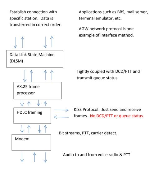
At the bottom we have the modem which sends digital bits through voice channels. The AX.25 protocol specification says absolutely nothing about the modems to be used. In practice we mostly use 1200 baud AFSK (based on Bell 202). For 9600 bps, it's really a two level baseband signal with pseudo random scrambling to reduce the DC component. This is often referred to as <u>G3RUH</u> for one of the early hardware designs.
