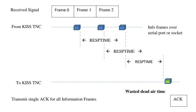
In this case, the link layer processing does not have access to the channel busy status. It doesn't know the radio channel speed, or PACLEN of the other station, to calculate the maximum frame time. How does it know when it has reached the last frame in the transmission? After each received frame comes along, wait RESPTIME before assuming no more frames are in the same transmission.
