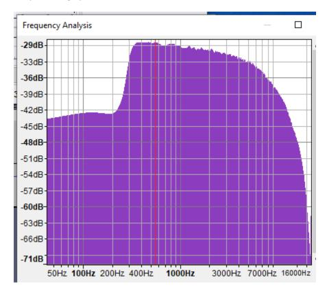
Maybe the control value is backwards. Let's enable the high pass filter and see if that turns it off. It looks essentially the same. So the highpass filter setting seems to be always on. Is it a bug in SA818-prog or the SA818?
