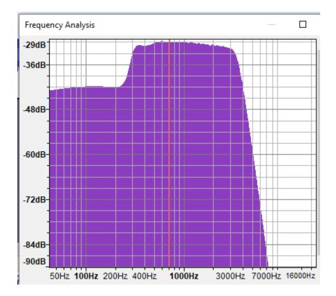
That is not what I expected at all. De-emphasis should decrease the signal by 6 dB per octave. That means half the amplitude when the frequency is doubled. Instead, we appear to have the highpass and lowpass filters. . Is it a bug in SA818-prog or the SA818?
