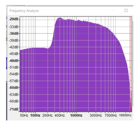
Now add the lowpass filter in addition to the highpass filter. I would expect this to attenuate frequencies over about 3 kHz which are not needed for voice. It seems to make no difference. Is it a bug in SA818-prog, or the SA818, or my misunderstanding?
