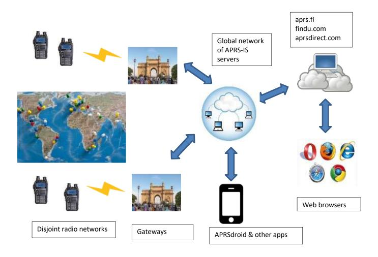
IGate stations allow communication between disjoint radio networks by allowing some content to flow between them over the Internet.
