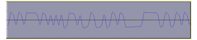
If high frequencies are attenuated, the nice square corners turn into overshoot and ringing. We don't reach the full amplitude when the signal is changing at the maximum rate (e.g. 4800 Hz square wave for 9600 baud). If the low frequencies are attenuated, the horizontal lines droop towards the middle shifting the zero reference level. There are system non-linearities especially if we are not centered in the FM discriminator bandpass. We can never escape the omnipresent noise.
