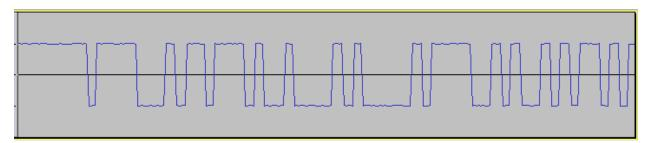
This is easy to decode. If the signal is positive, call it a logic 1. If negative, call it a logic 0.
