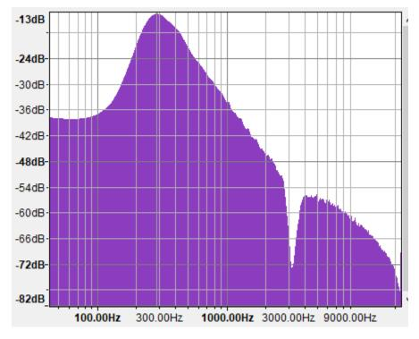
We notice that higher frequencies are being attenuated at about -12 dB per octave rather than the expected -6 dB per octave. There is also a huge notch just above 3 kHz.
