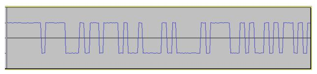
On the receiving end, we use a digital phase locked loop (DPLL), synchronized to the zero crossings, to determine where to sample for the data bits.
