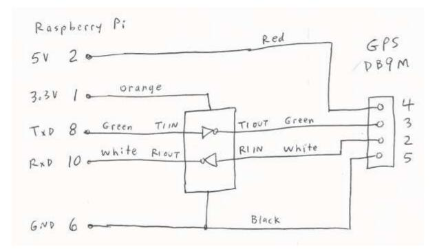
5 volts, to power the GPS, is supplied through pin 4. This is the same convention commonly used by other trackers such as OpenTrack and Tiny Trak4 so the same GPS receiver should be interchangeable between them.
